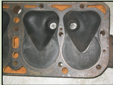
'Police Head' high compression combustion chamber with a compression ratio of 5.22 to 1.
