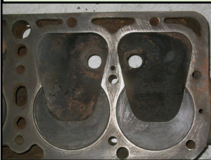
Stock Model A cylinder head combustion chamber with compression ratio of 4.22 to 1.
