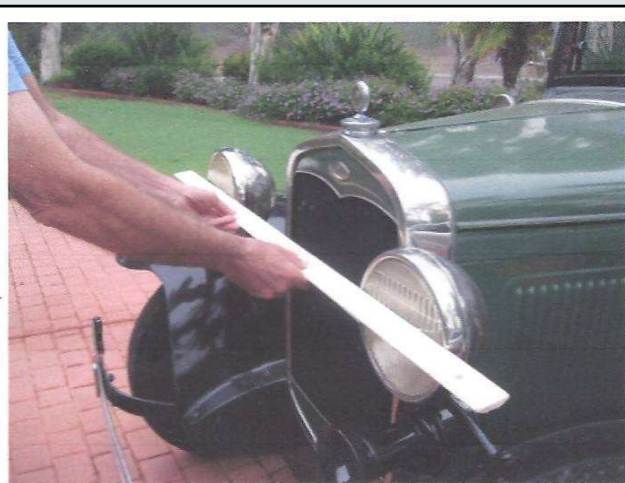
Adjust so that both lights are flat against the straight edge.
