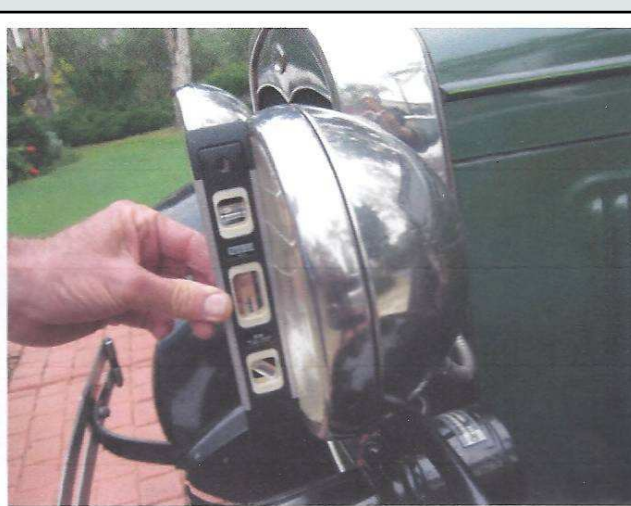
Adjust lights for 1/2 bubble forward tilt.
