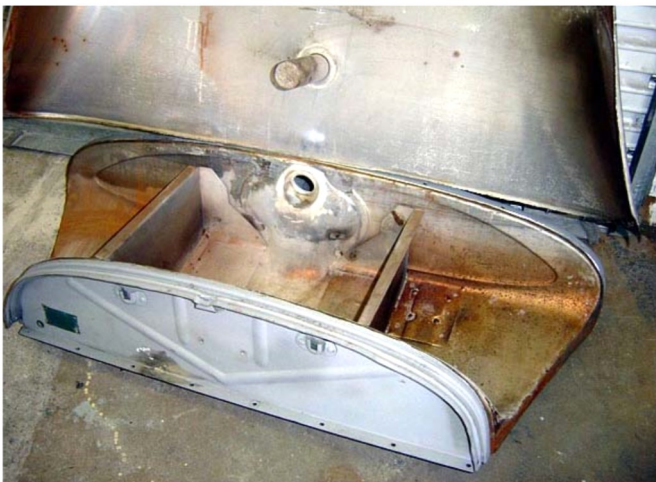
28-29 Gas Tank Cut Open
