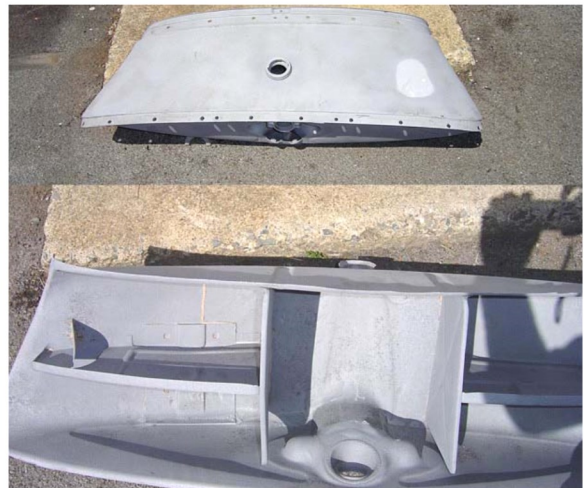
30-31 Gas Tank Cut Open
