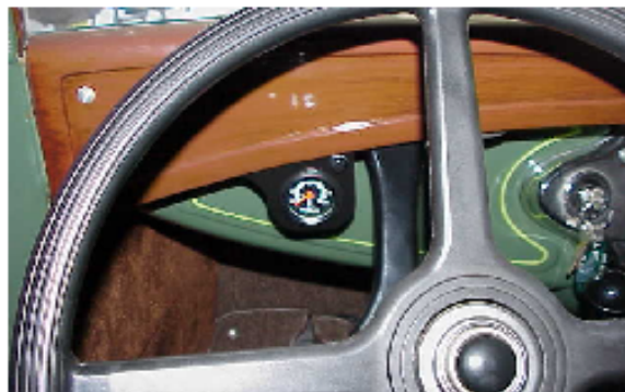
A 1 1/2-inch SunPro mechanical temperature gauge is installed with a custom made bracket up under the dash rail of a 1931 Victoria.
