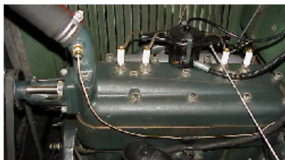
The six-foot mechanical cable is routed from the gauge to the Dan Eubanks reproduction water outlet casting that has been cast with a temp gauge boss and has been drilled and tapped for your favorite size pipe fitting. Dan locates the fitting on the side of the casting to accommodate an overhead valve head installation. (Dan Eubanks 626-827-4004).
