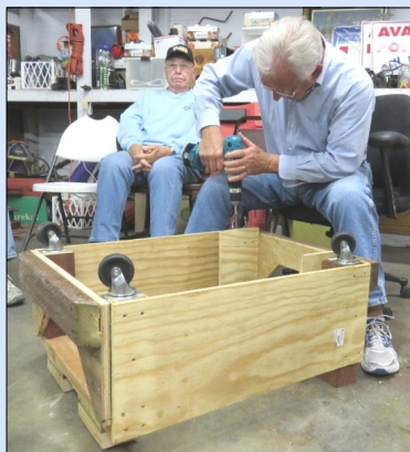
Jim doing extensive caster reconfiguration on engine dolly
