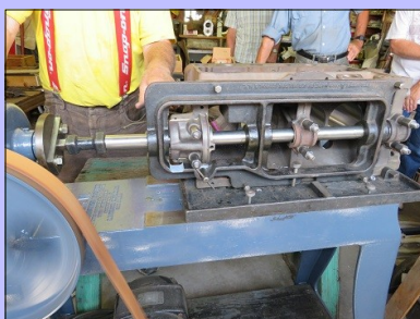
Boring tooling set-up
