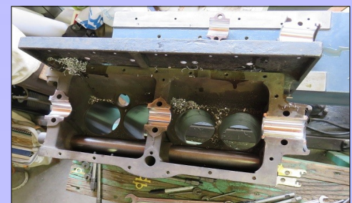
Boring completed. Ready for reaming-to-size operation
