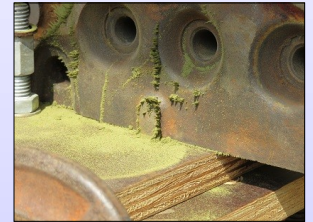
Cracks revealed with magnafluxing
