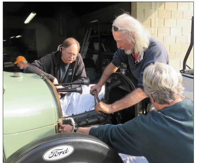
Gary torquing head after gasket replacement. Steve and Monty supervising. . .
