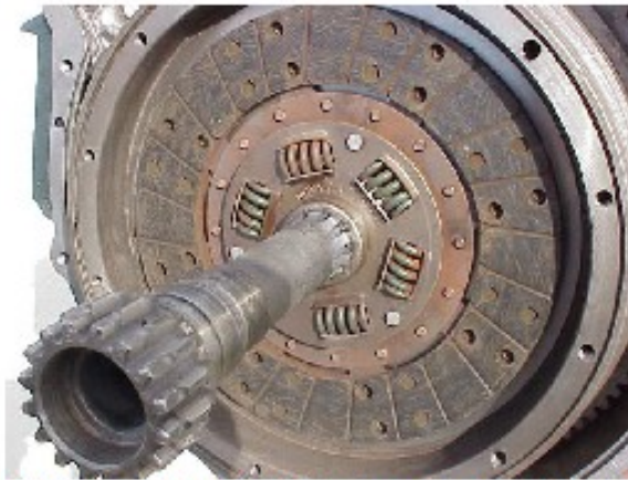
A Nova clutch disk: Note how each of the six springs are secured by a flange top and bottom. Flanges are installed on the backside as well.
