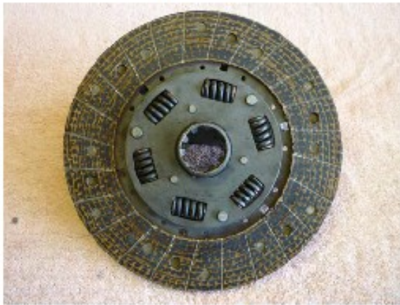
The six springs are not well secured. They can easily become dislodged.
