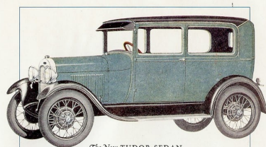
The New TUDOR SEDAN Long, wide, roomy. Narrow pillars and new door construction give unusual room. Both front seats fold forward, giving easy access to rear seat. Ample space between seats.
